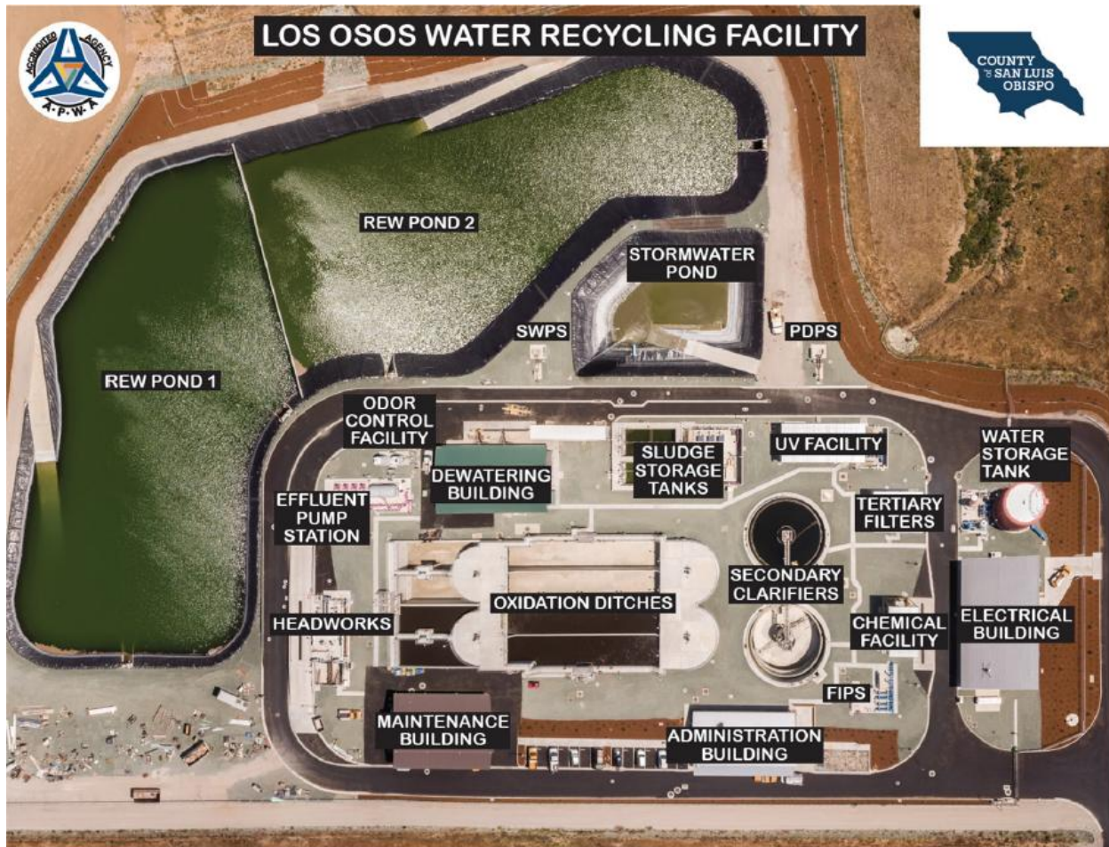
Figure 3-2. Los Osos Water Recycling Facility Site Map
