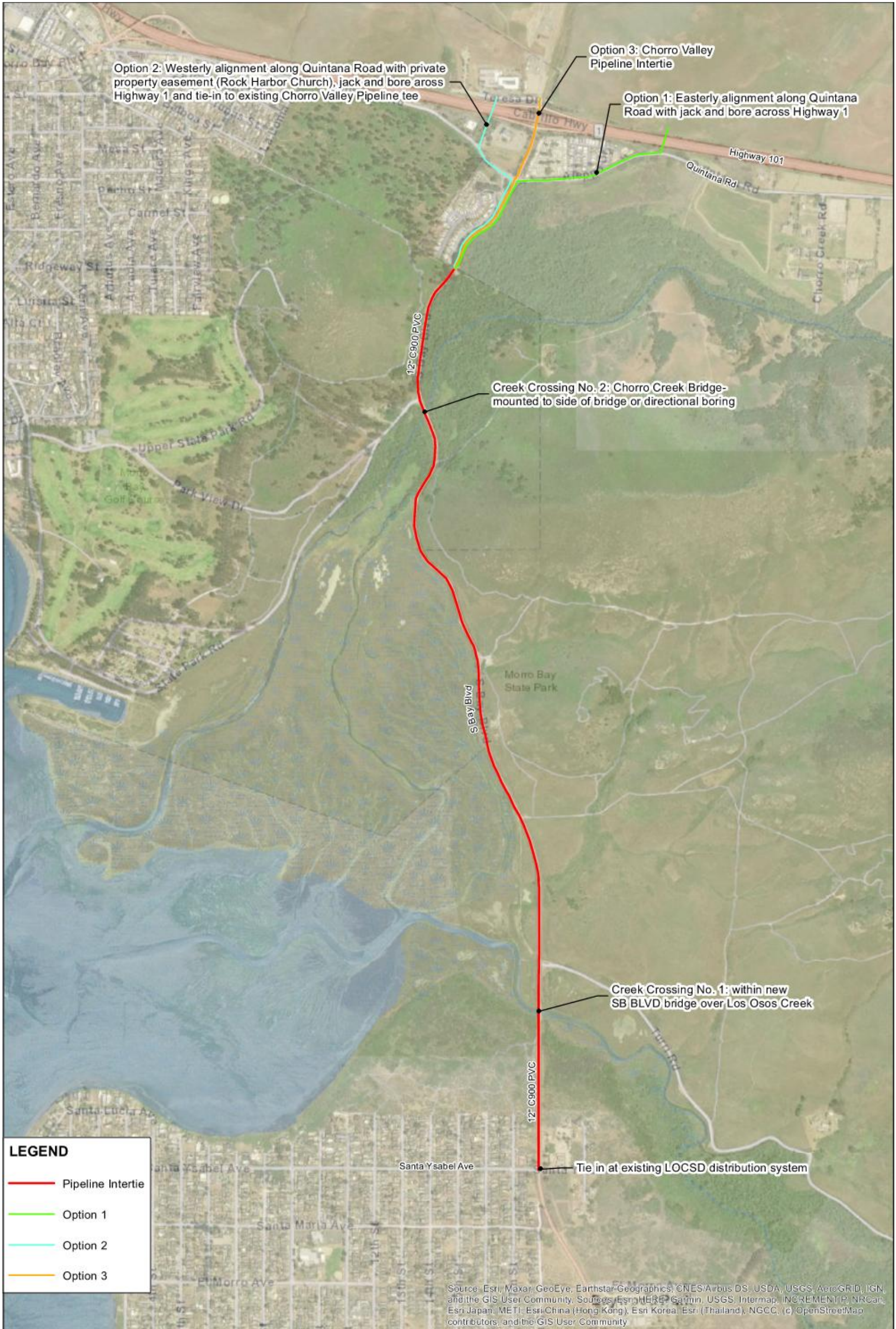
Figure 5-15. Possible Water Resiliency Intertie Pipeline Alignments
